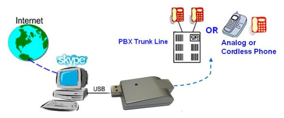
Connect SkyATA with analog PBX trunk line or analog phone
